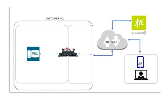
In this case, connectivity will be done using a trunk group registered and pointing to Jive Virtual Service, and connected in the back end with an IPPBX.
