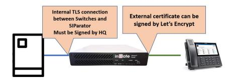
Interface eth0 (Inside) will have a certificate signed by HQ Server as explained in Create an HQ signed certificate to be used in the SIParator® internal interface for TLS.
